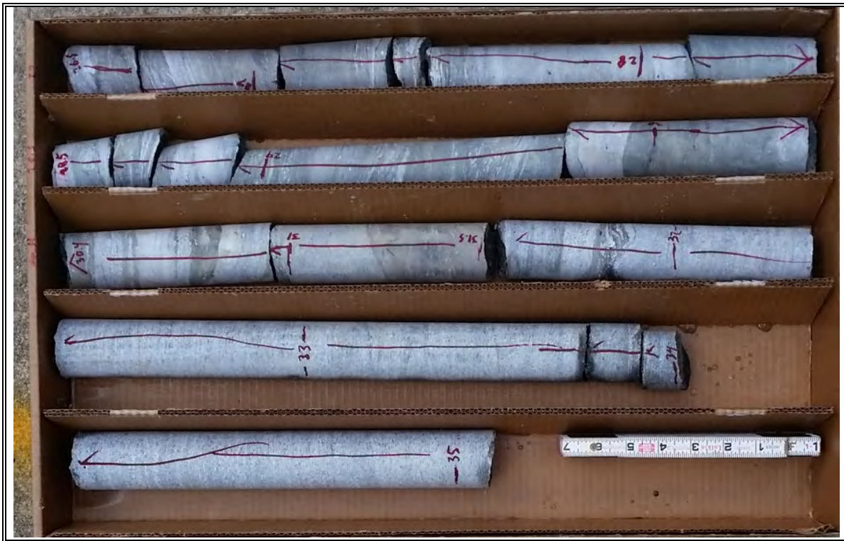
Rock Core from HM-5 (26.5' – 35.0') Run 1: REC= 100% RQD = 84.2% Run 2: REC= 100% RQD = 92.8%
