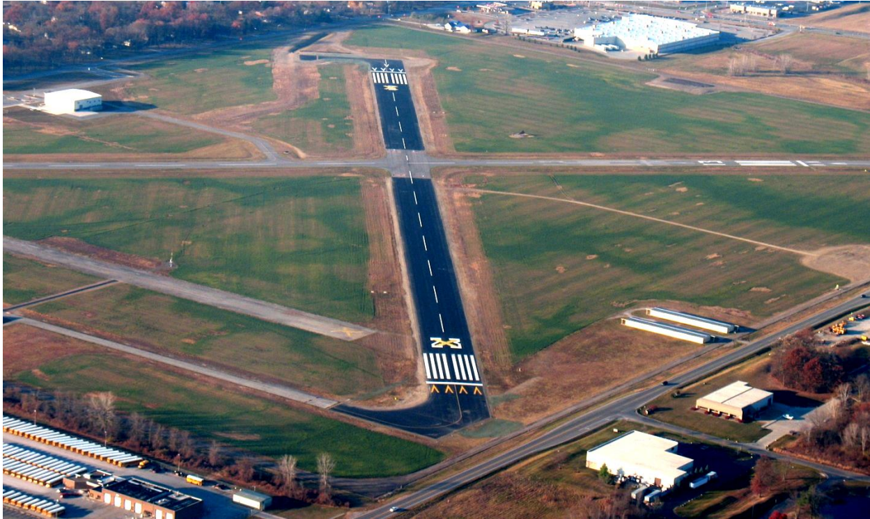
Figure 2-3. Markings for a Temporarily Closed Runway
