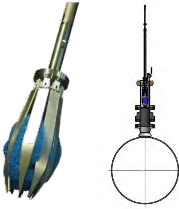
Figure 4.1: Insertion Tool (left) and Stack Setup (right)
