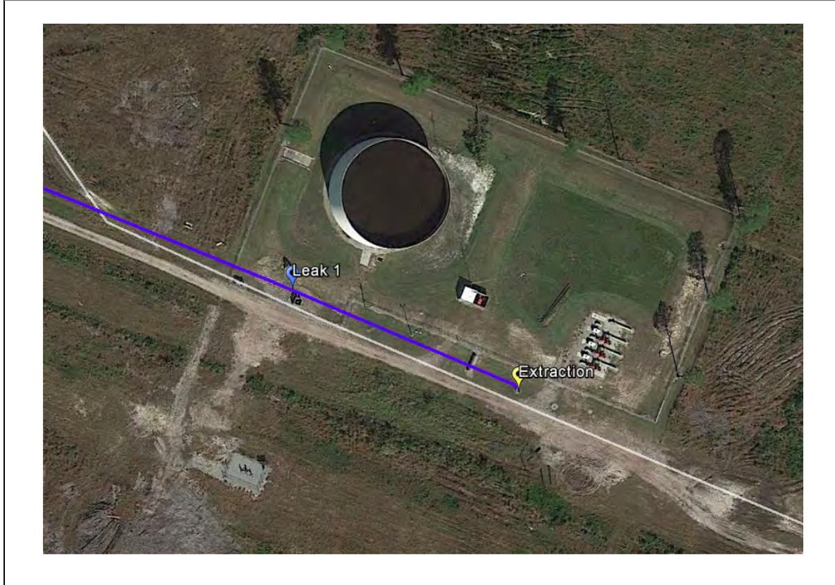
The location and small size of the detected anomaly leads to the conclusion that the suspected leak could be a valve seated incorrectly. The location lines up with the valve from the raw water main to the ground storage tank adjacent to the LCFWSA Interim Booster Station site. It is advised that this valve be worked to ensure it is operating and sitting correctly. If the valve is functioning properly the location should be investigated further to determine the source of the detected leak.
