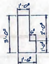
PRECAST CONCRETE L-BEAM 60H-P STRAND PATTERN
