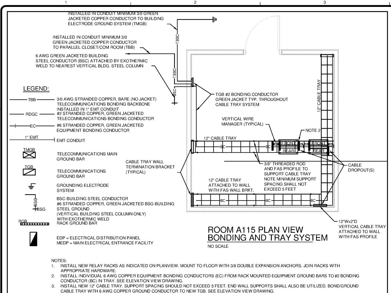
4. INSTALL #2 COPPER BONDING CONDUCTOR (BC) INTO THE LENGTH OF NEW CABLE TRAY, ORIGINATING AT TGB. TAPE ALL BARE ENDS AND BONDS.
