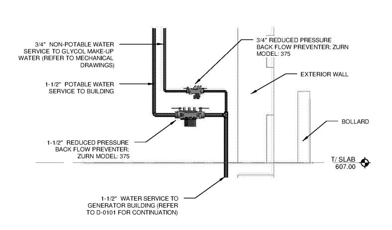
REDUCED PRESSURE BACK FLOW P-8101 SCALE: N.T.S.
