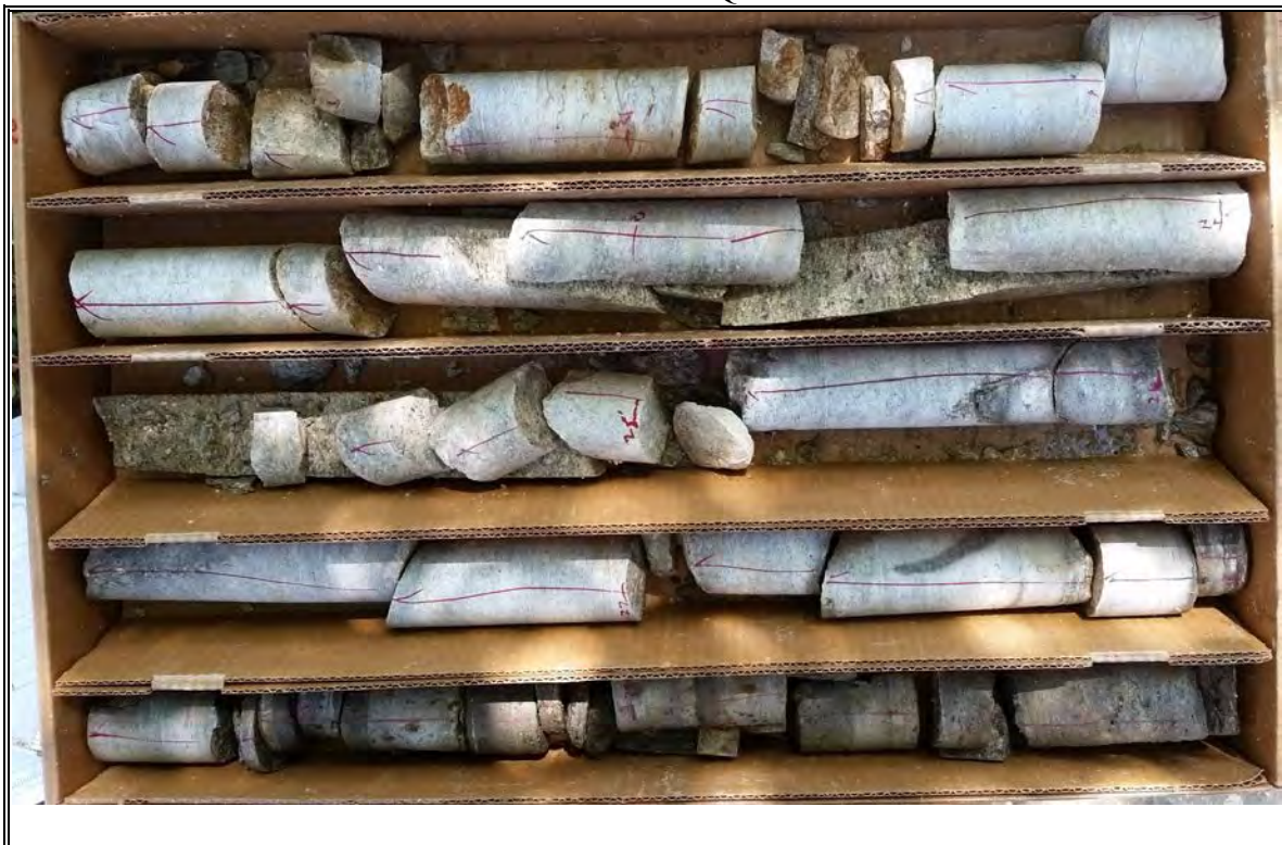
Rock Core from HM-6 (20.0' - 30.0') Run 1: REC=100% RQD =21.7% Run 2: REC=100% RQD =38.3%
