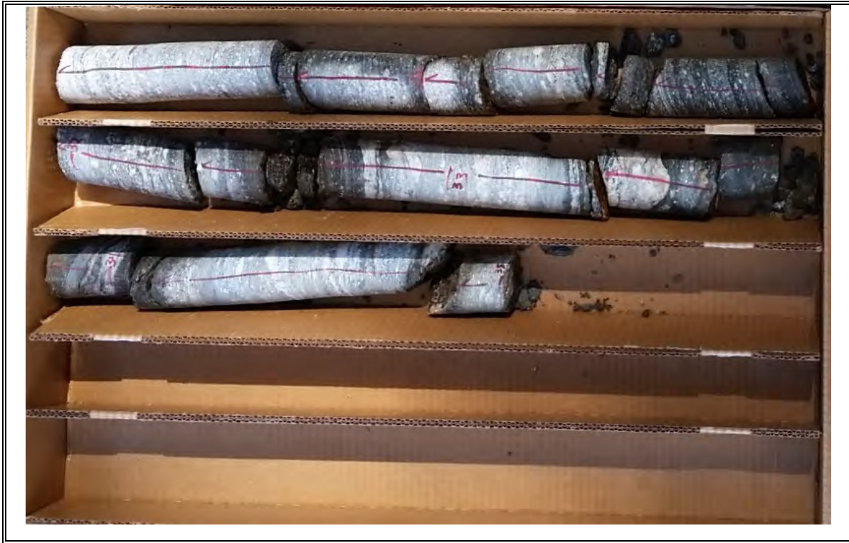
Rock Core from HM-9 (30.0' – 35.0') Run 1 : REC=100% RQD=60%
