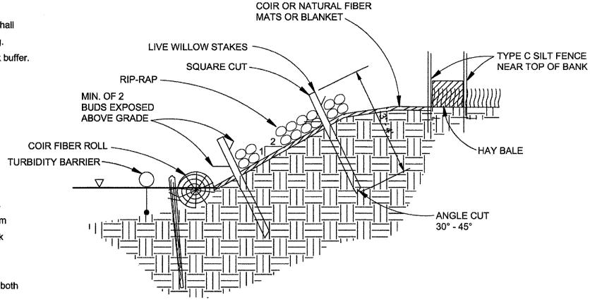
LIVE WILLOW STAKE INSTALLATION NOTES: 1. The live willow stakes should be tamped into the ground at right angles to the slope and angled downstream. They should be tamped
