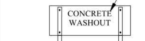
CONCRETE WASHOUT SIGN DETAIL
