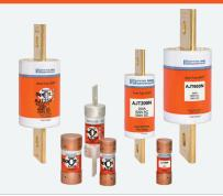
Amp-Trap 2000® AJT fuses provide non-indication as well as a SmartSpot® visual open fuse indicator. With advanced material technology the AJT fuse provides IEC Type 2 No Damage protection to main, feeder, and branch circuits, for all types of loads — yet, they require only half the mounting space needed for 600VAC Class RK fuses. AJT's time-delay characteristics are ideal for handling typical motor and transformer inrush currents, while also providing superior current-limiting ability.
