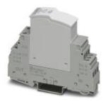
Pluggable device protection, according to type 3/class III, for 1-phase power supply networks with separate N and PE (3-conductor system: L1, N, PE), with integrated surge-proof fuse and remote indication contact. Also suitable for DC applications.
