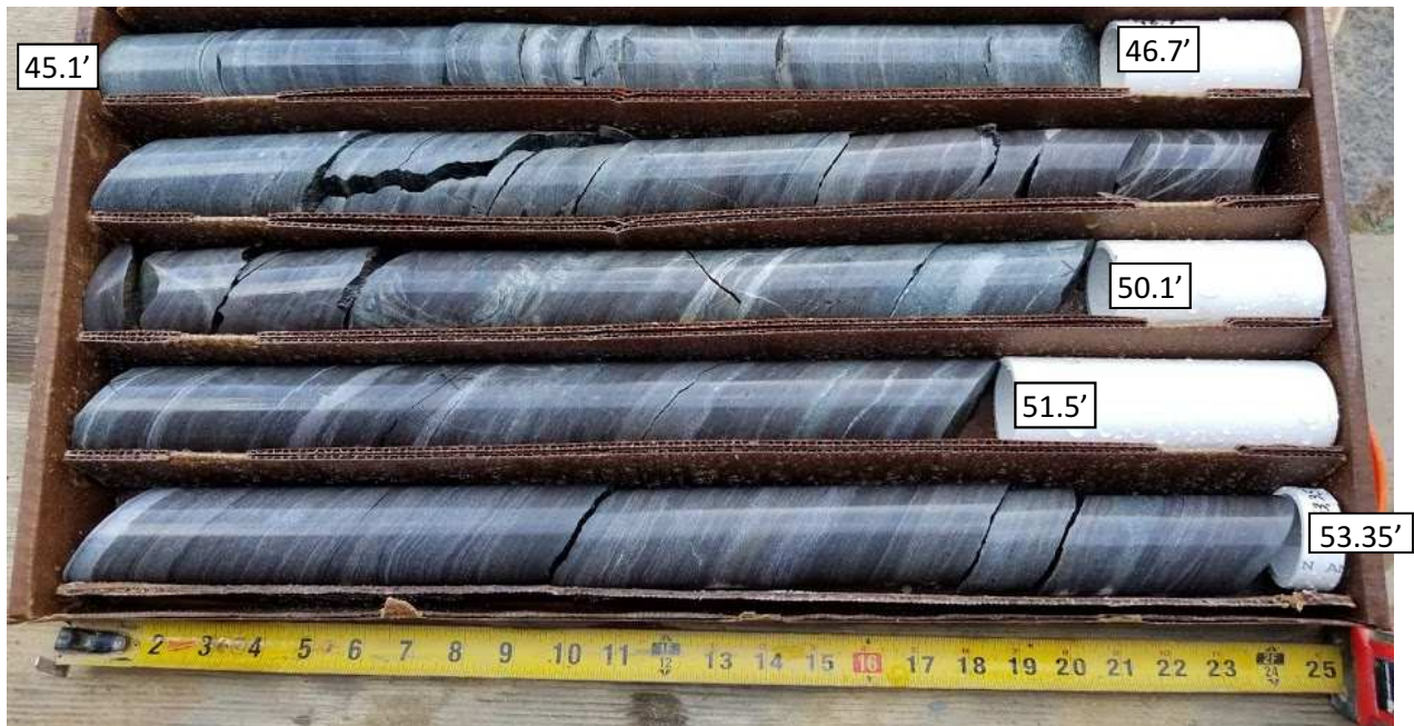
SPT-1A Core Run #7: 44-49 ft bgs REC = 100%, RQD = 34%
