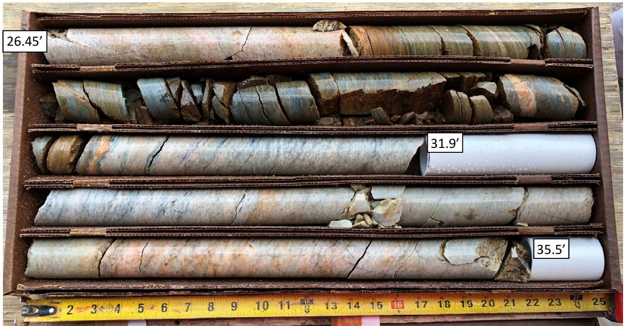
SPT-1A Core Run #3: 24-29 ft bgs REC = 100%, RQD = 48%
