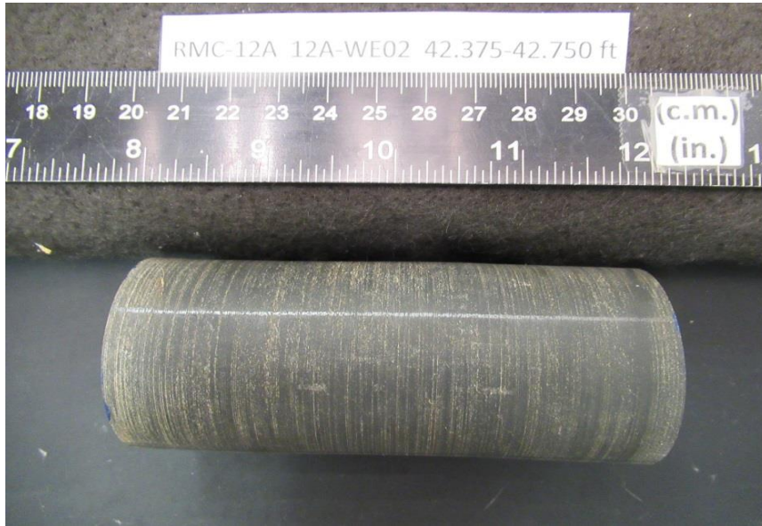
After cutting and grinding
