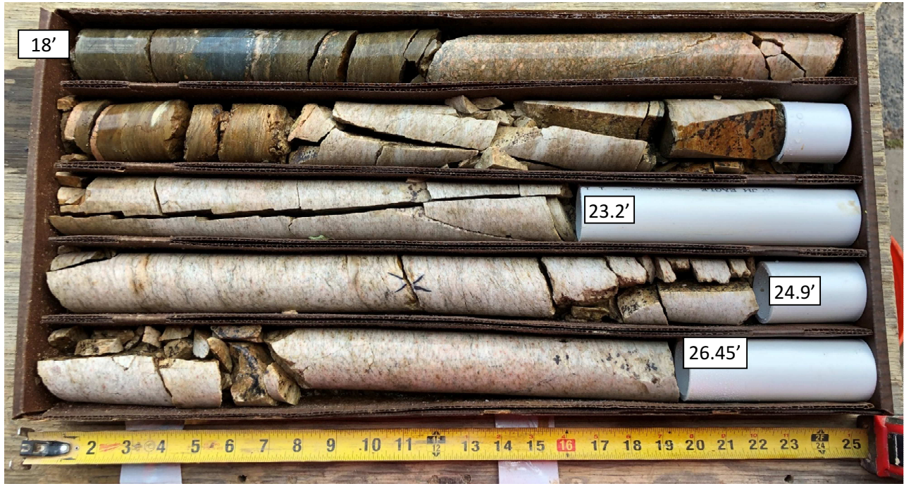
SPT-1A Core Run #1: 18-19 ft bgs REC = 90%, RQD = 45%
