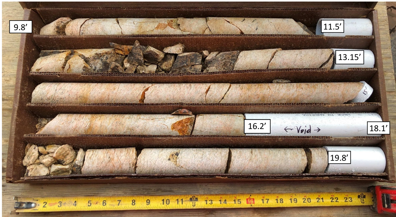
SPT-2A Core Run #1: 9.8-19.8 ft bgs REC = 81%, RQD = 41%
