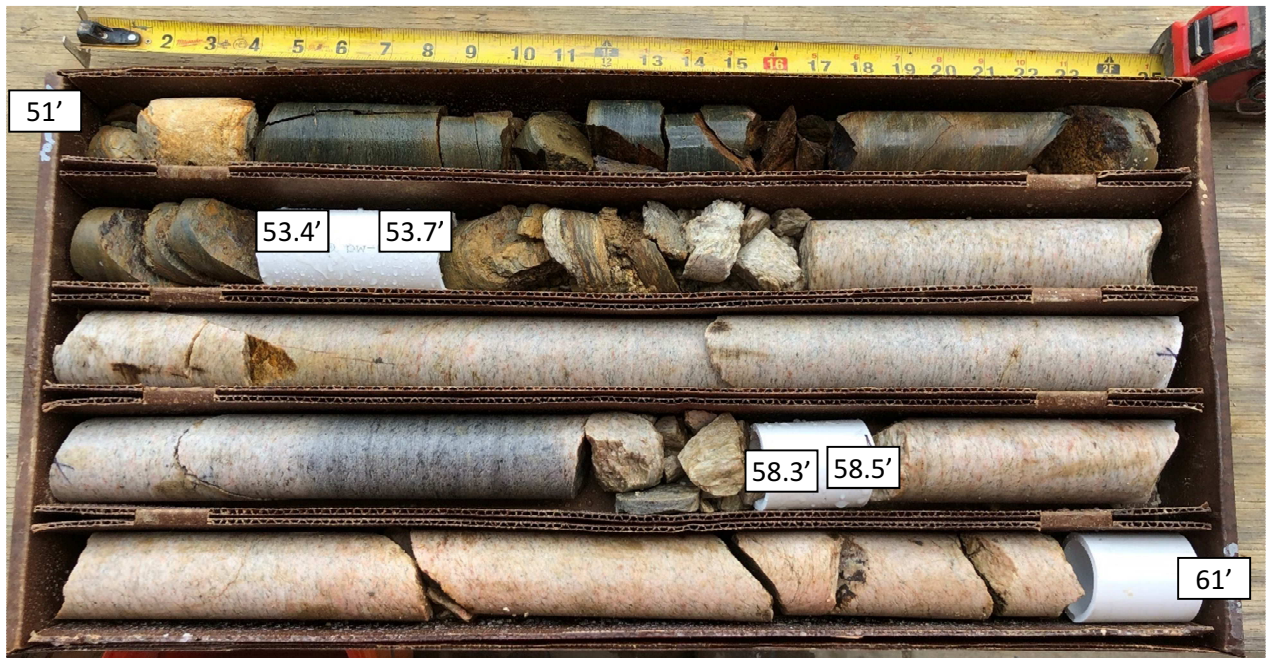
GC-1A Core Run #2: 51-61 ft bgs REC = 93%, RQD = 58%
