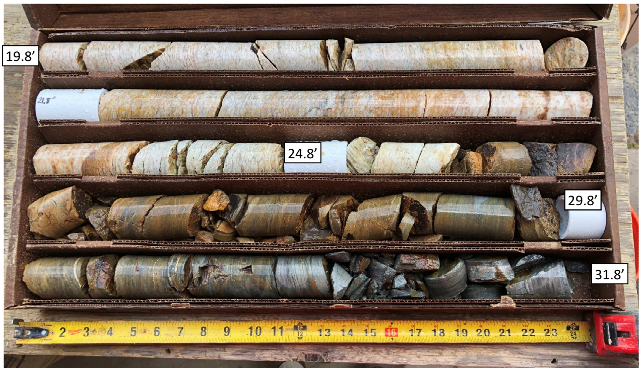
SPT-2A Core Run #2: 19.8-29.8 ft bgs REC = 74%, RQD = 26%
