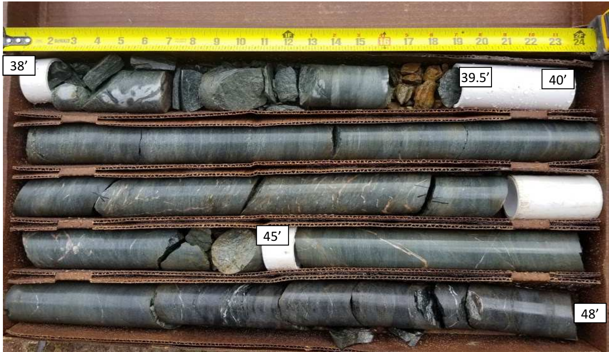
SPT-6A Core Run #3: 35-45 ft bgs REC = 77%, RQD = 52%
