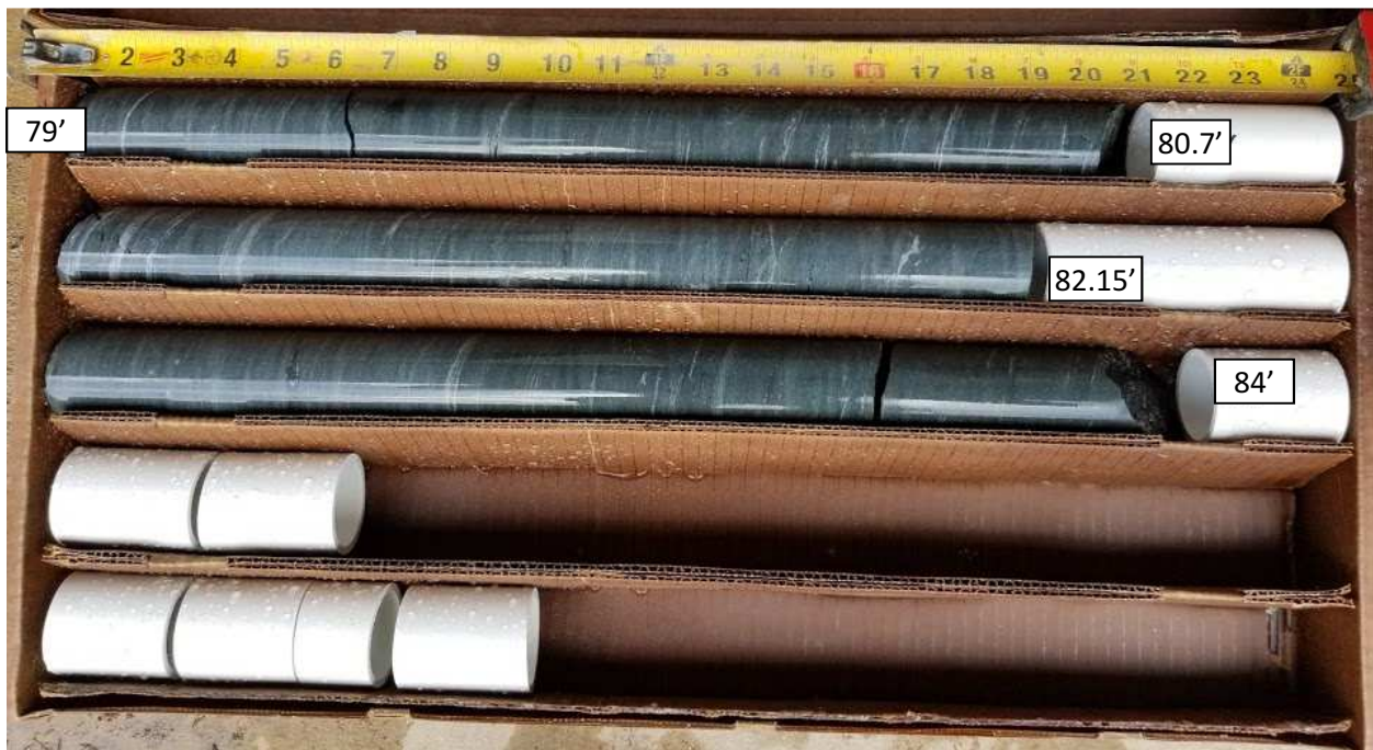
SPT-1A Core Run #14: 79-84 ft bgs REC = 100%, RQD = 100%
