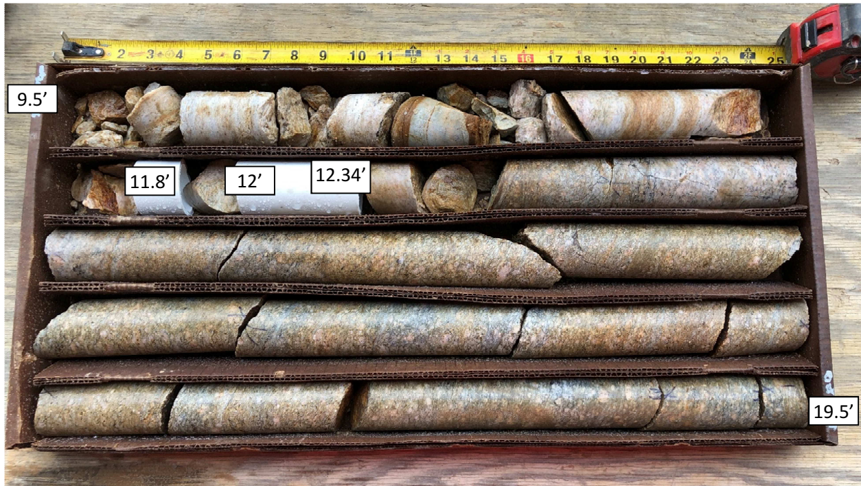
GC-2A Core Run #1: 9.5-19.5 ft bgs REC = 95%, RQD = 74%
