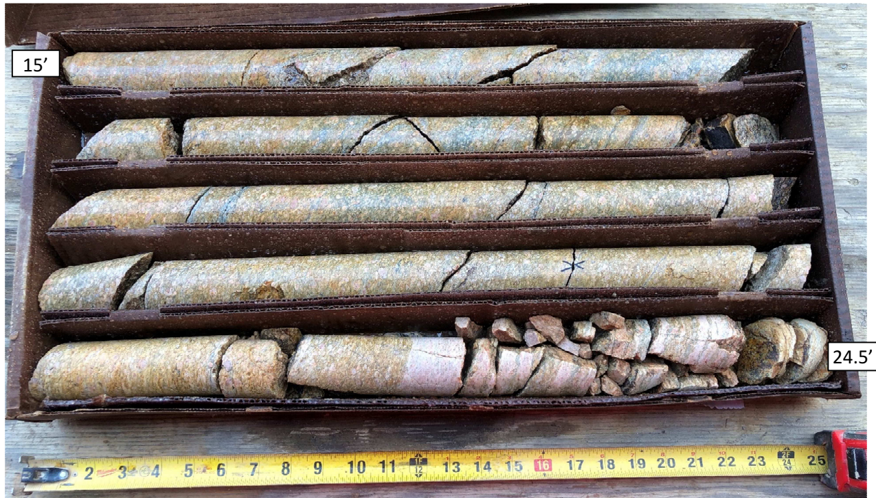
SPT-10B Core Run #1: 15-25 ft bgs REC = 100%, RQD = 65%
