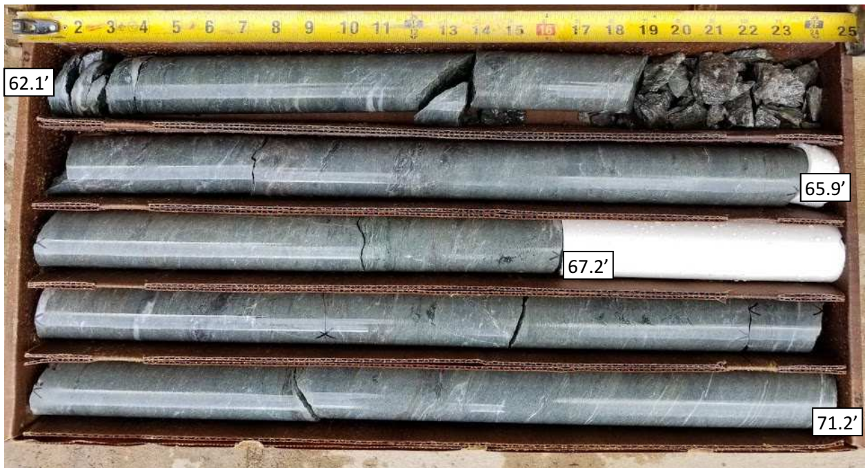
SPT-1A Core Run #11: 64-69 ft bgs REC = 100%, RQD = 100%
