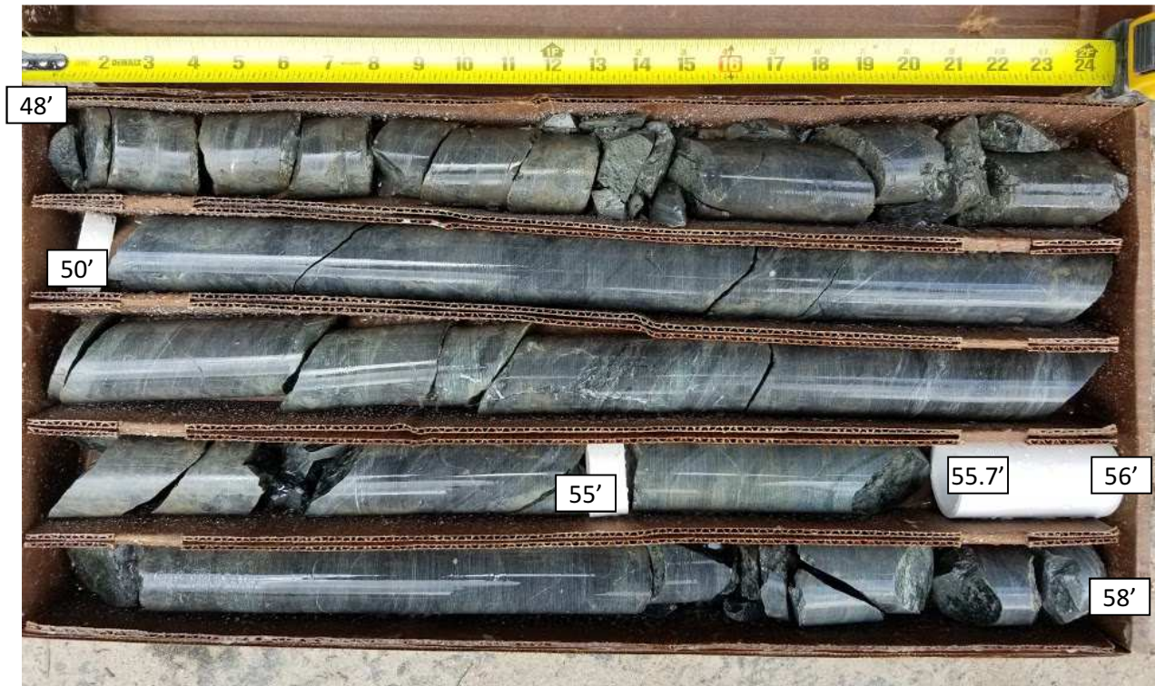
SPT-6A Core Run #4: 45-55 ft bgs REC = 100%, RQD = 78%
