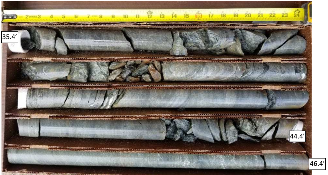
SPT-5A Core Run #2: 35.4-44.4 ft bgs REC = 86%, RQD = 53%
