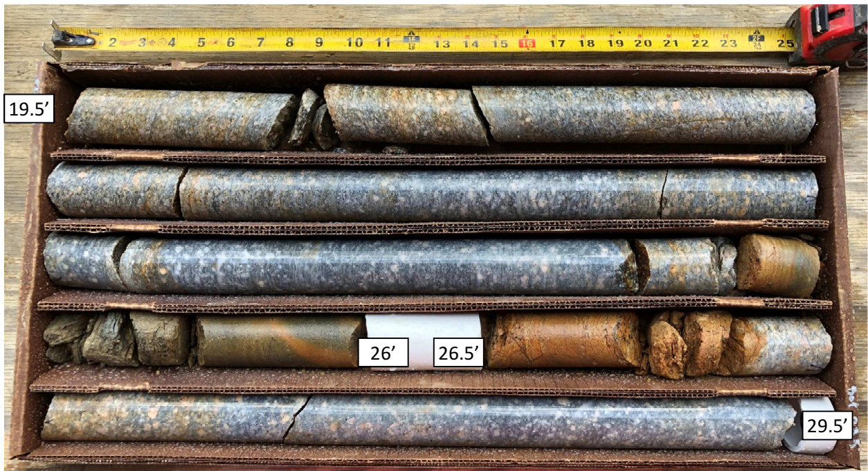
GC-2A, Core Run #2: 19.5-29.5 ft bgs REC = 96%, RQD = 83%
