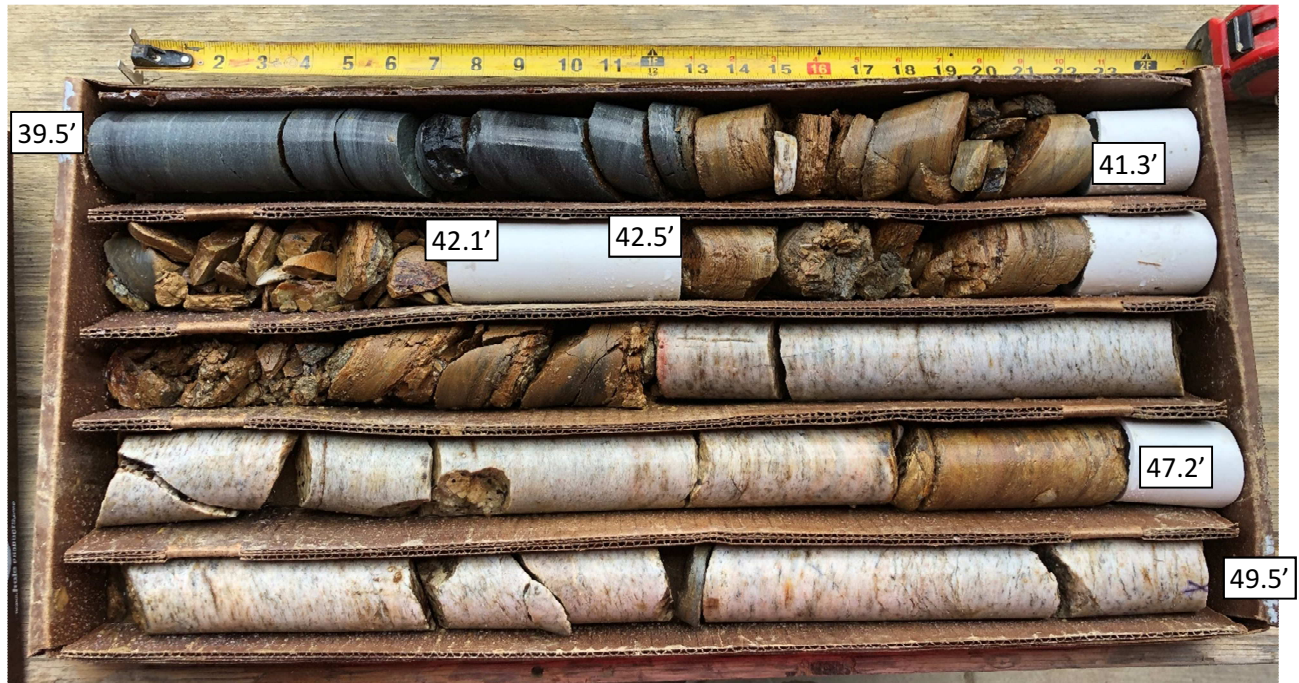
GC-2A Core Run #4: 39.5-49.5 ft bgs REC = 91%, RQD = 38%
