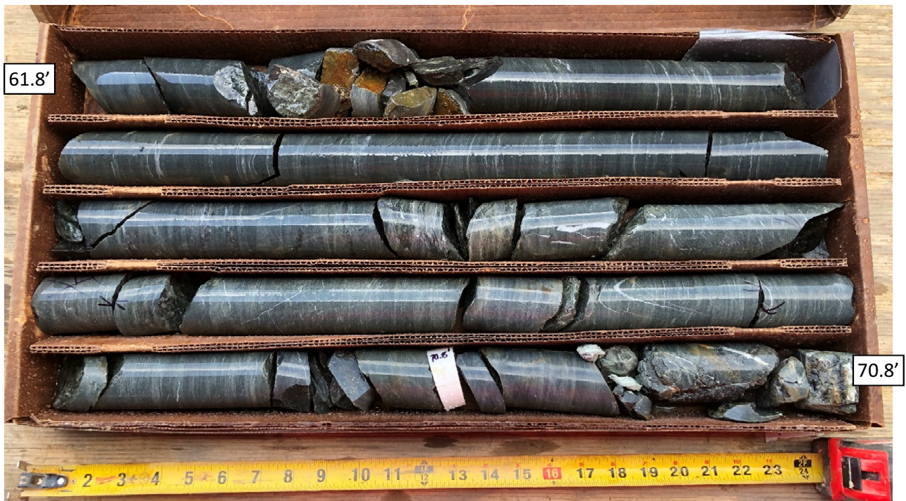
SPT-2A Core Run #6: 59.8-71.8 ft bgs REC = 100%, RQD = 76%
