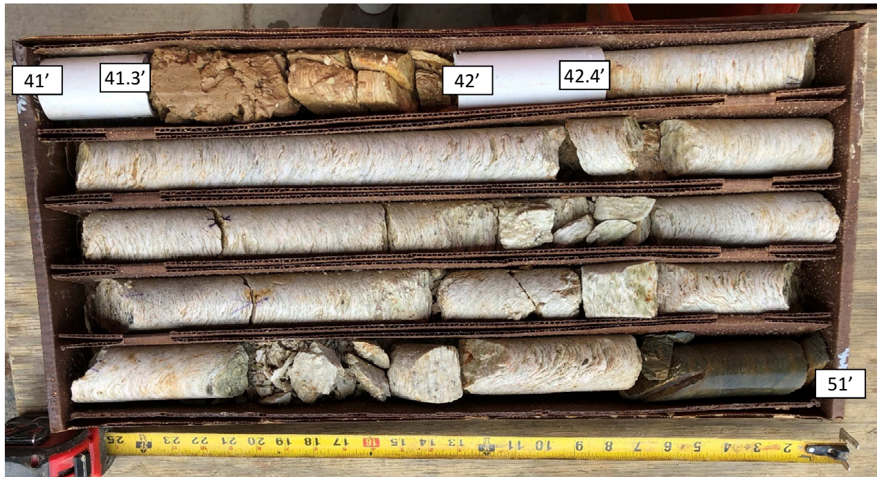
GC-1A Core Run #1: 41-51 ft bgs REC = 94%, RQD = 63%
