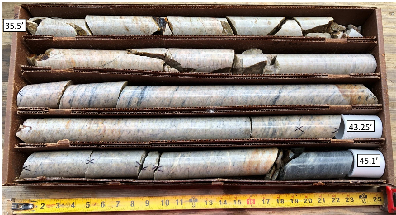
SPT-1A Core Run #5: 34-39 ft bgs REC = 100%, RQD = 32%
