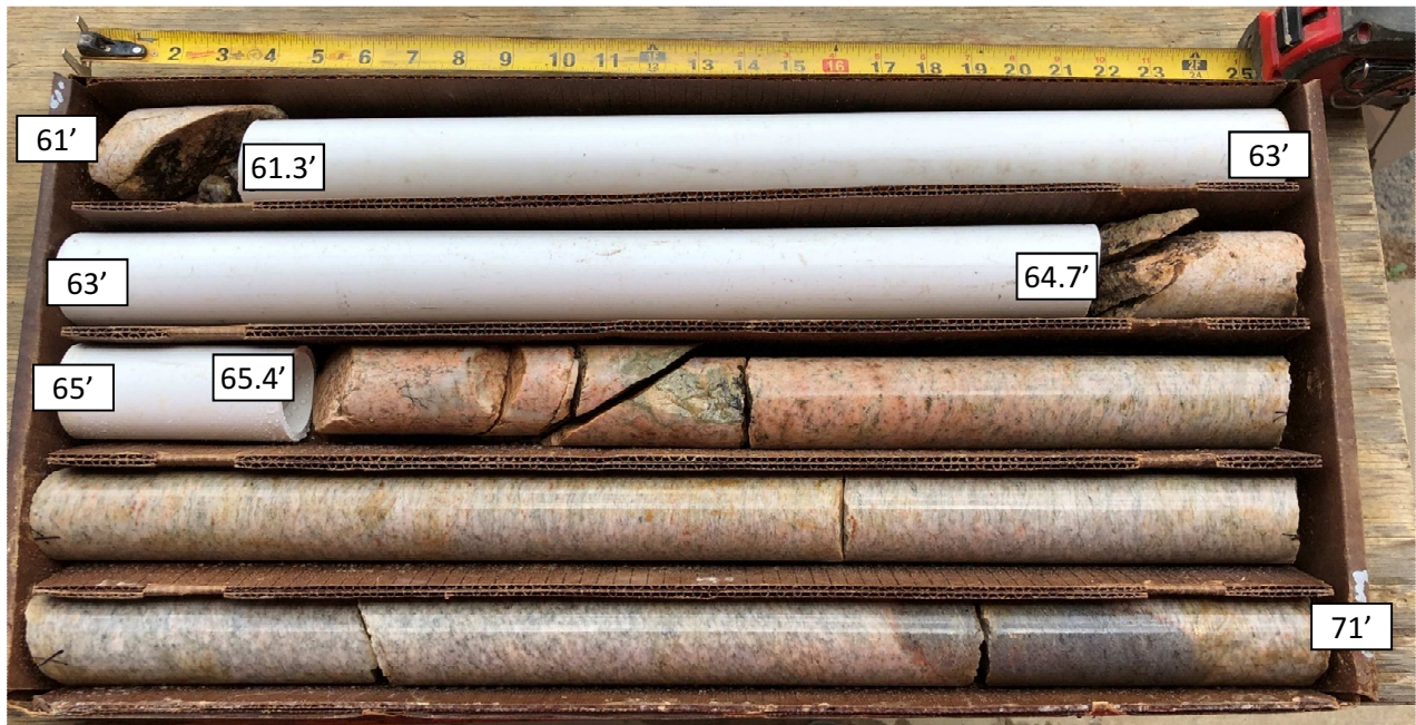
GC-1A Core Run #3: 61-71 ft bgs REC = 63%, RQD = 49%
