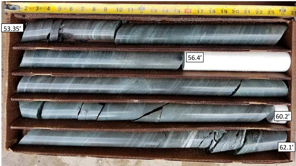
SPT-1A Core Run #9: 54-59 ft bgs REC = 100%, RQD = 88%
