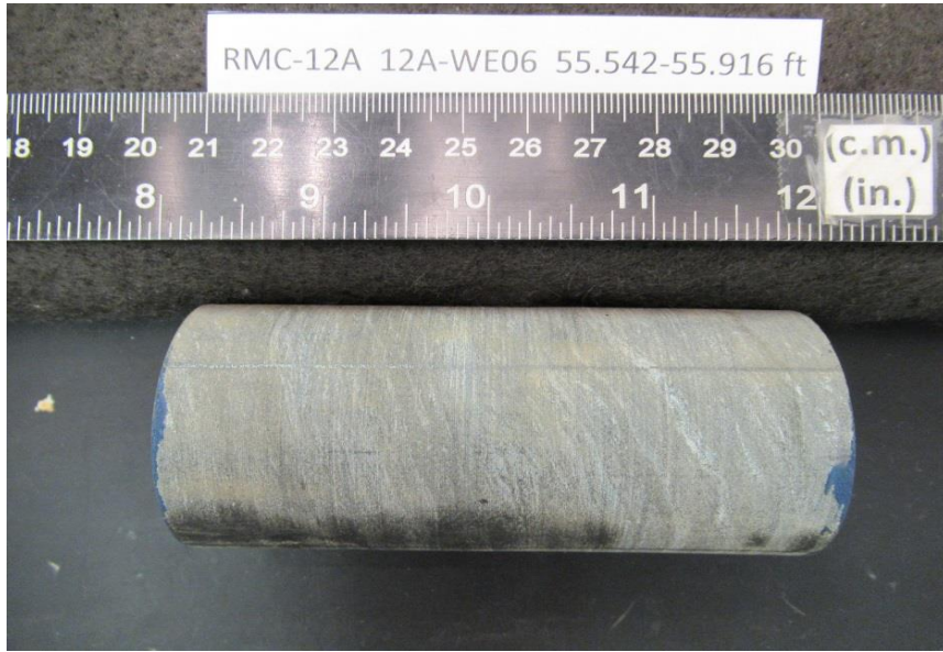
After cutting and grinding
