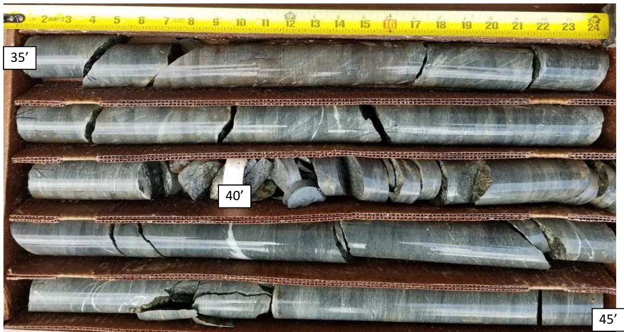
SPT-4A Core Run #2: 35-45 ft bgs REC = 100%, RQD = 83%
