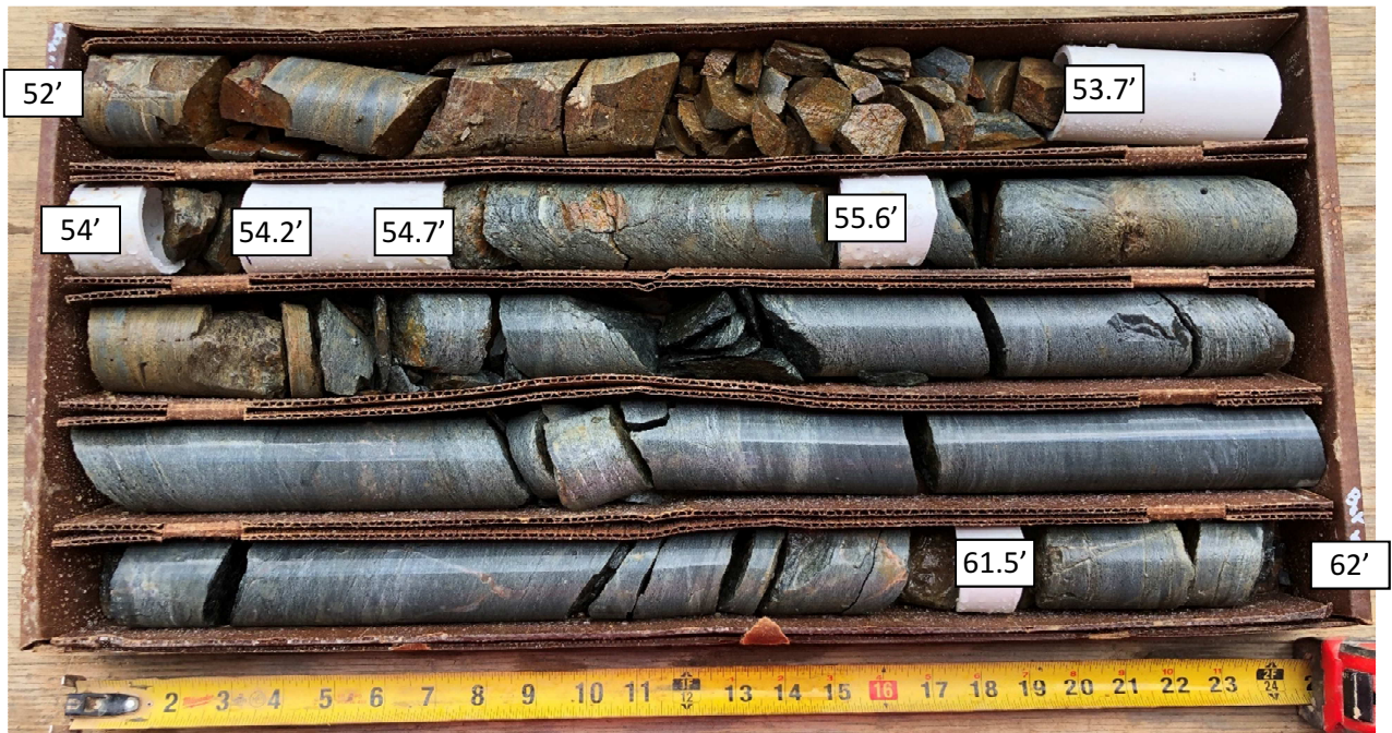
SPT-3A Core Run #3: 52-62 ft bgs REC = 89%, RQD = 41%
