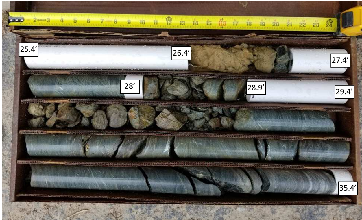
SPT-5A Core Run #1: 25.4-35.4 ft. bgs REC = 74%, RQD = 40%
