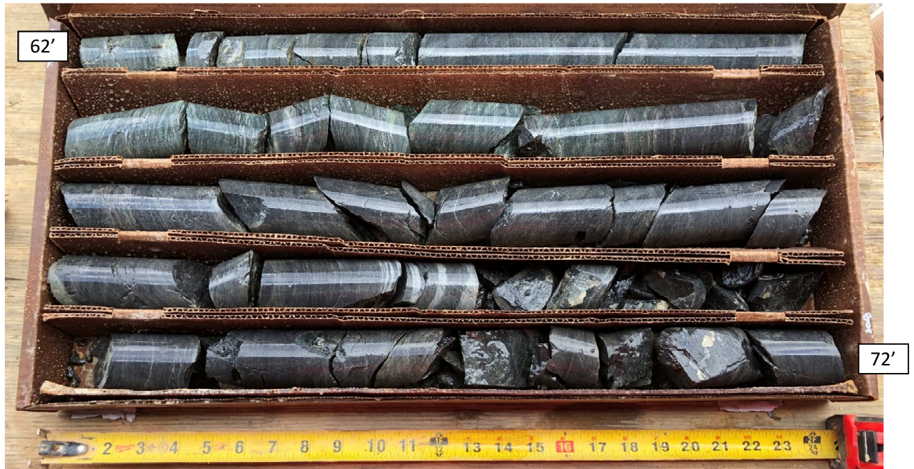
SPT-3A Core Run #4: 62-72 ft bgs REC = 100%, RQD = 38%
