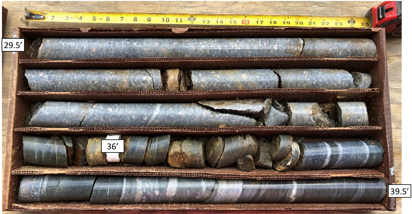
GC-2A Core Run #3: 29.5-39.5 ft bgs REC = 99%, RQD = 73%
