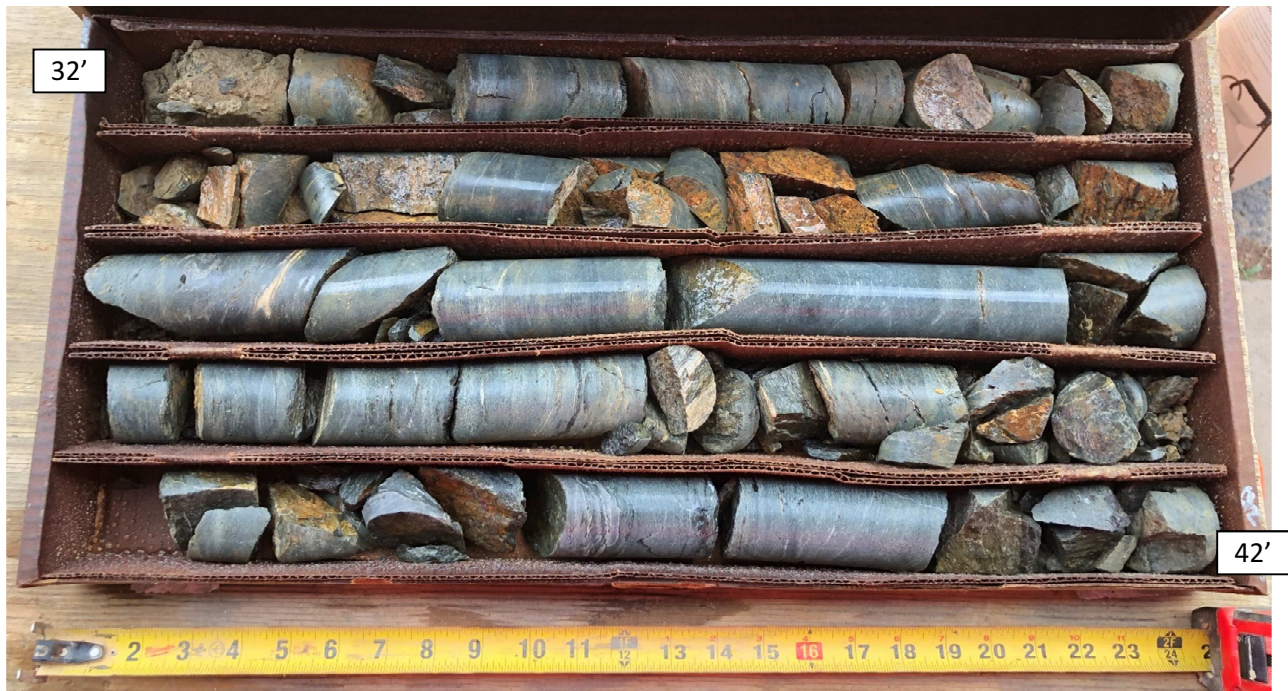
SPT-3A Core Run #1: 32-42 ft bgs REC = 95%, RQD = 29%
