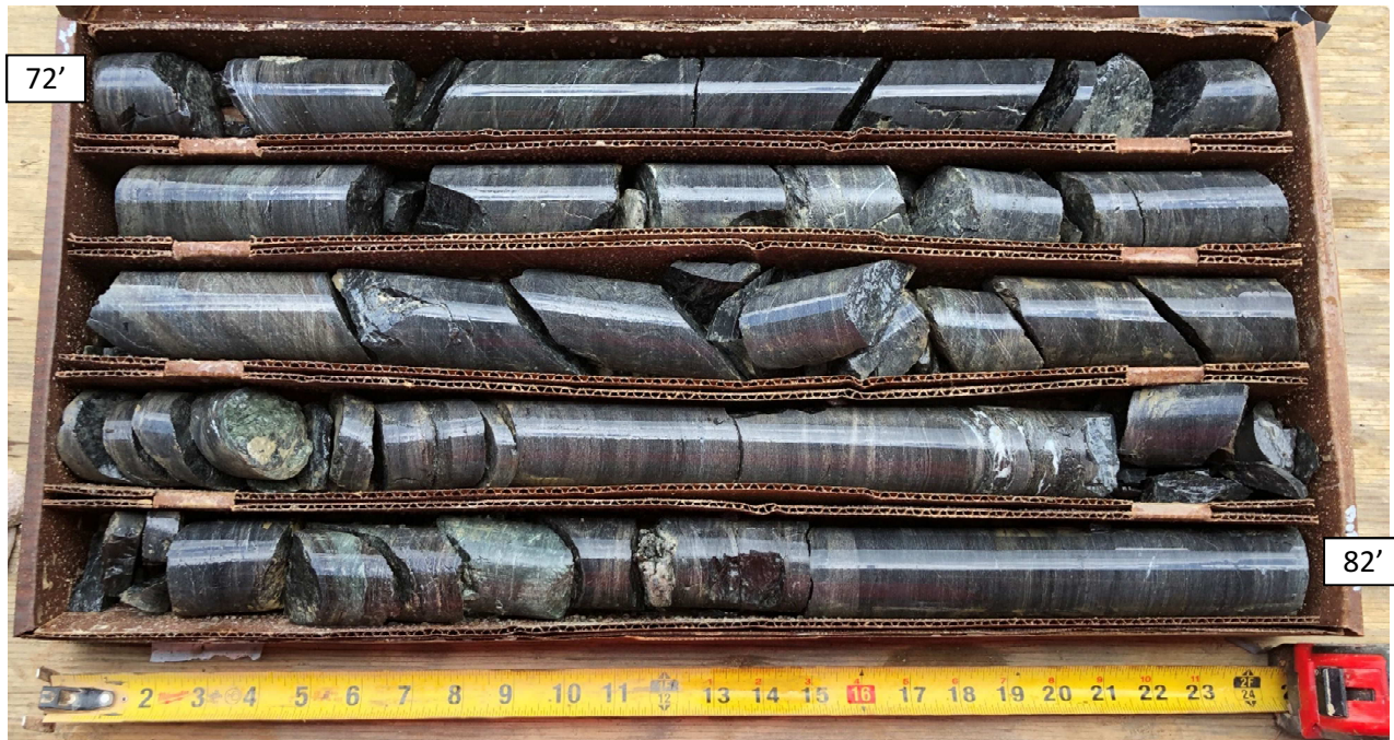
SPT-3A Core Run #5: 72-82 ft bgs REC = 100%, RQD = 35%
