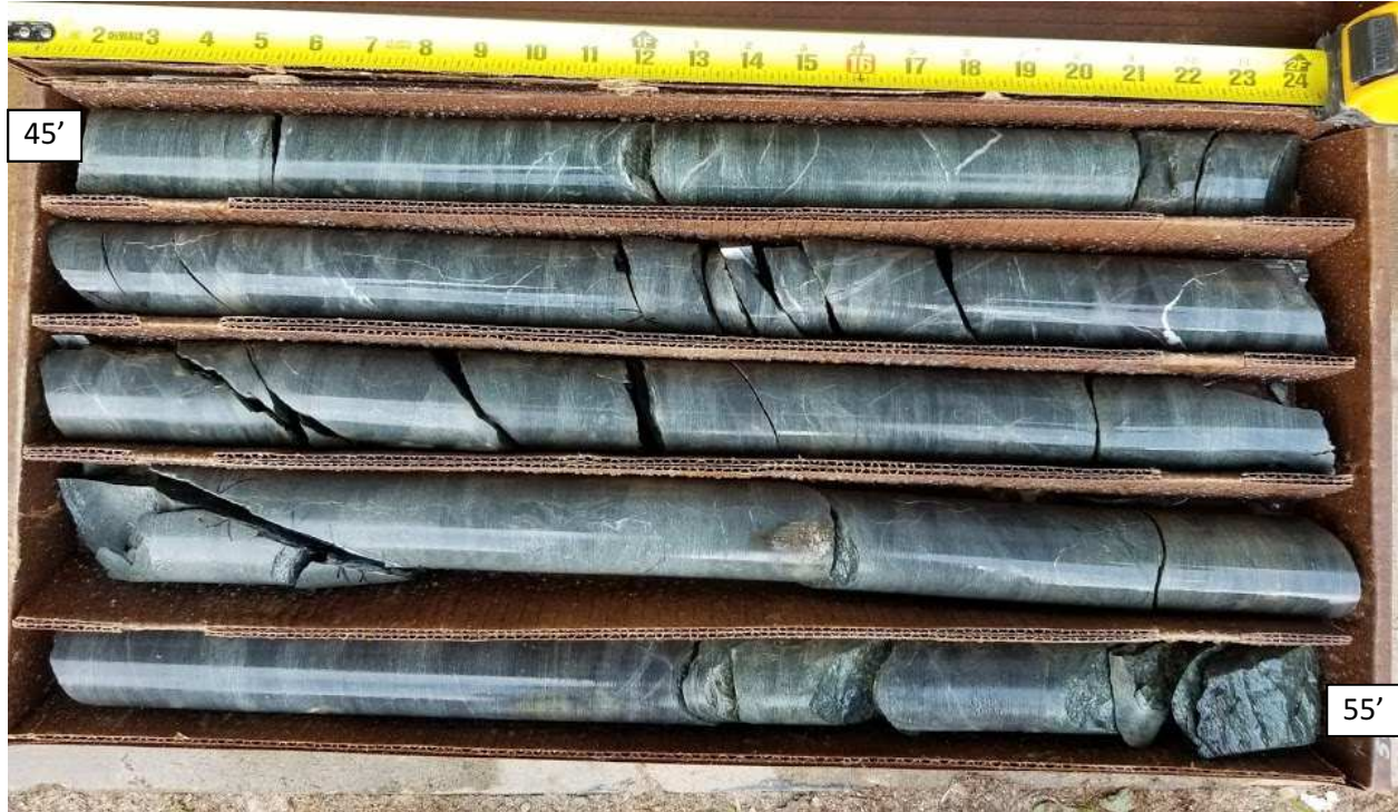
SPT-4A Core Run #3: 45-55 ft bgs REC = 100%, RQD = 78%
