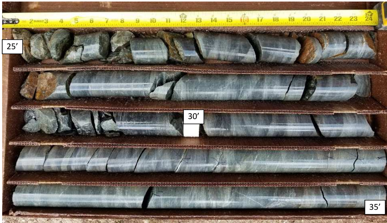
SPT-4A Core Run #1: 25-35 ft bgs REC = 95%, RQD = 59%
