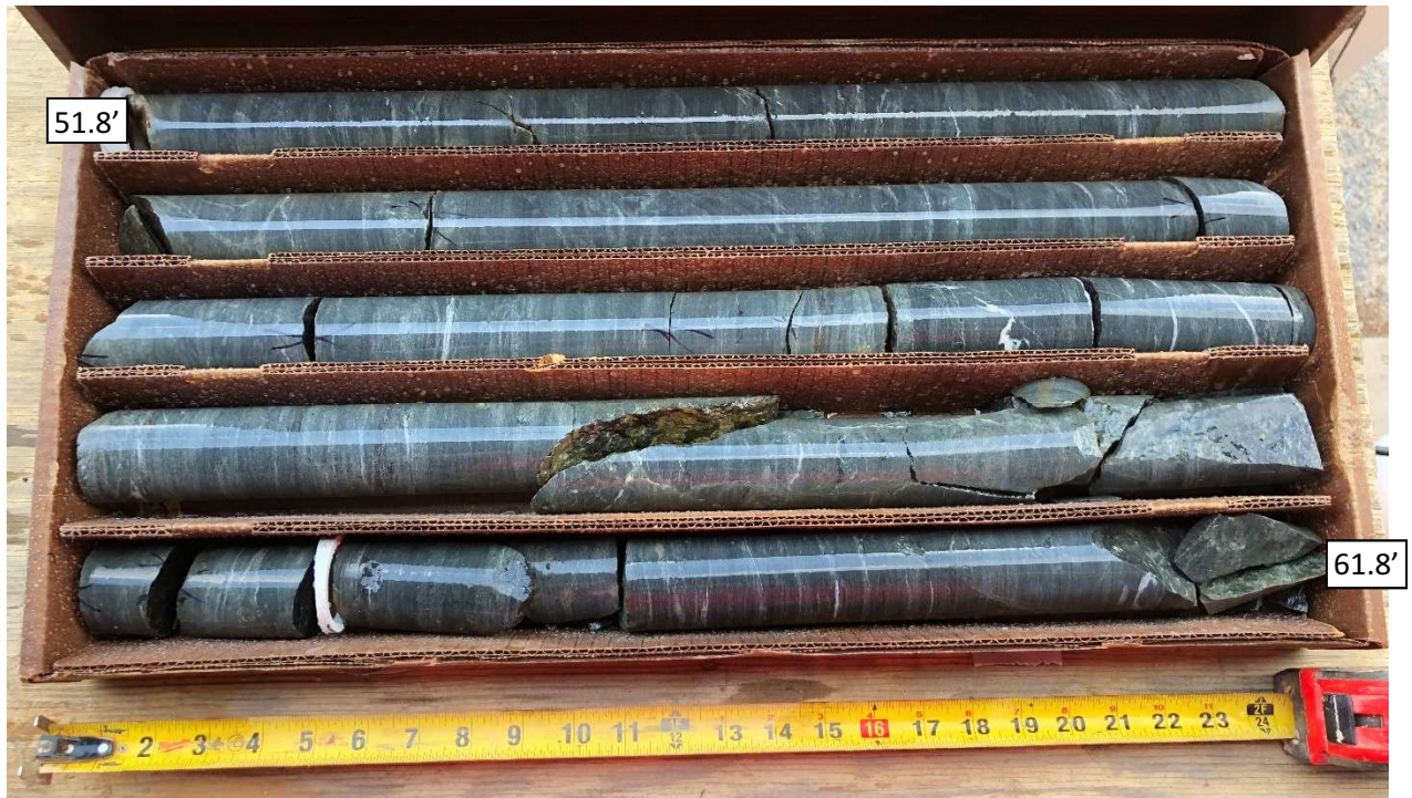
SPT-2A Core Run #5: 49.8-59.8 ft bgs REC = 100%, RQD = 100%
