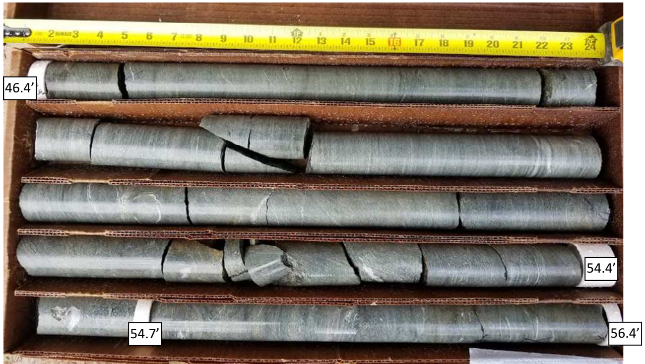
SPT-5A Core Run #3: 44.4-54.4 ft bgs REC = 99%, RQD = 94%
