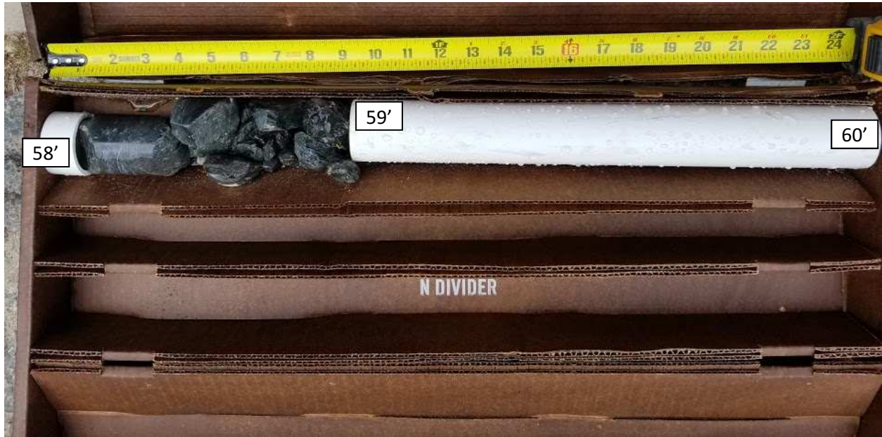
SPT-6A Core Run #5: 55-59 ft bgs REC = 82%, 39%
