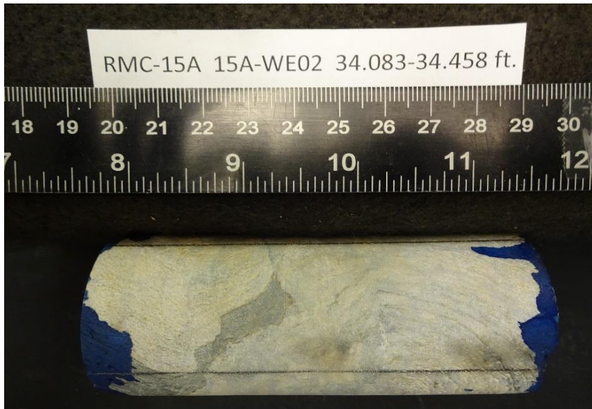
After cutting and grinding
