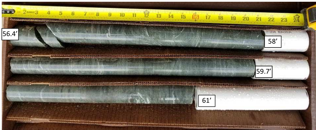
SPT-5A Core Run #4: 54.4-61 ft bgs REC = 100%, RQD = 99%
