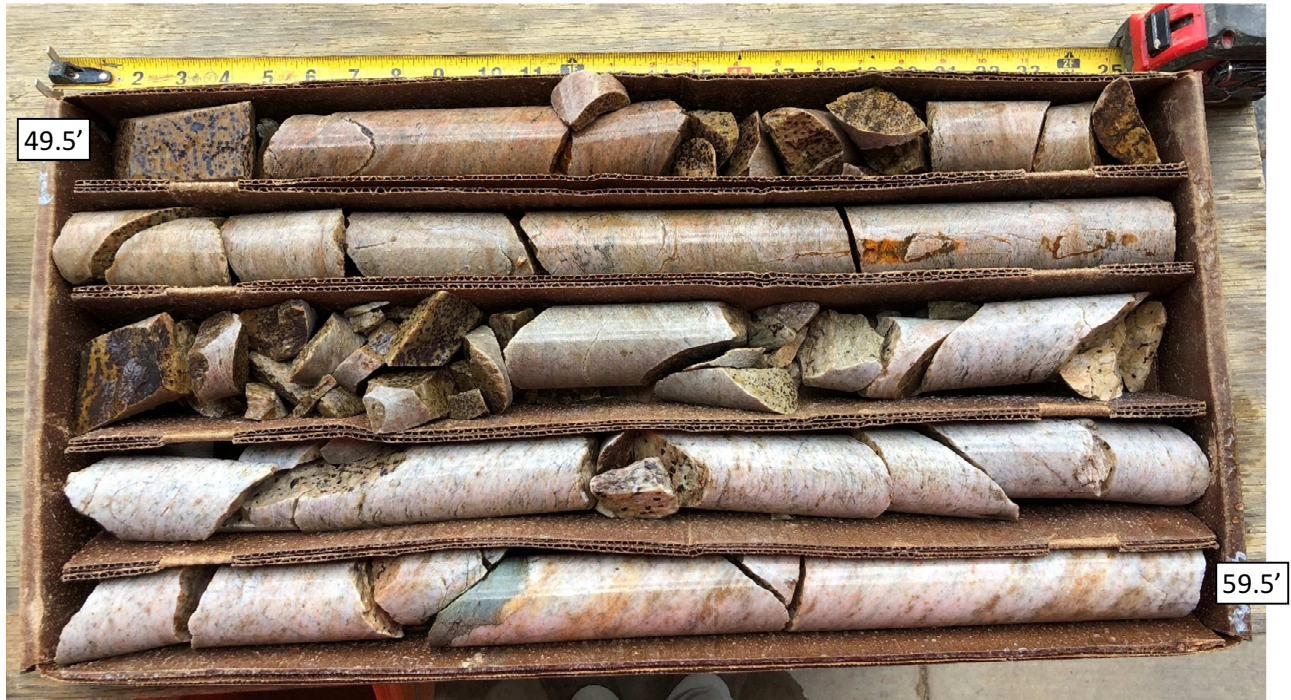
GC-2A Core Run #5: 49.5-59.5 ft. bgs REC = 100%, RQD = 57%
