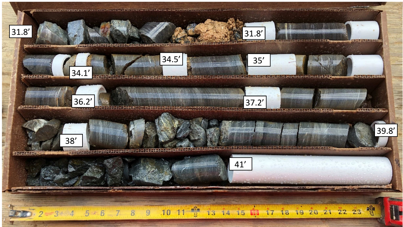
SPT-2A Core Run #3: 29.8-39.8 ft bgs REC = 85%, RQD = 15%
