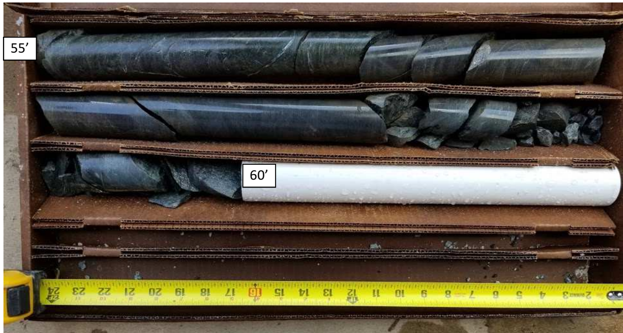
SPT-4A Core Run #4: 55-60 ft bgs REC = 93%, RQD = 58%
