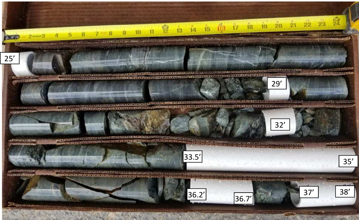
SPT-6A Core Run #2: 25-35 ft bgs REC = 80%, RQD = 51%
