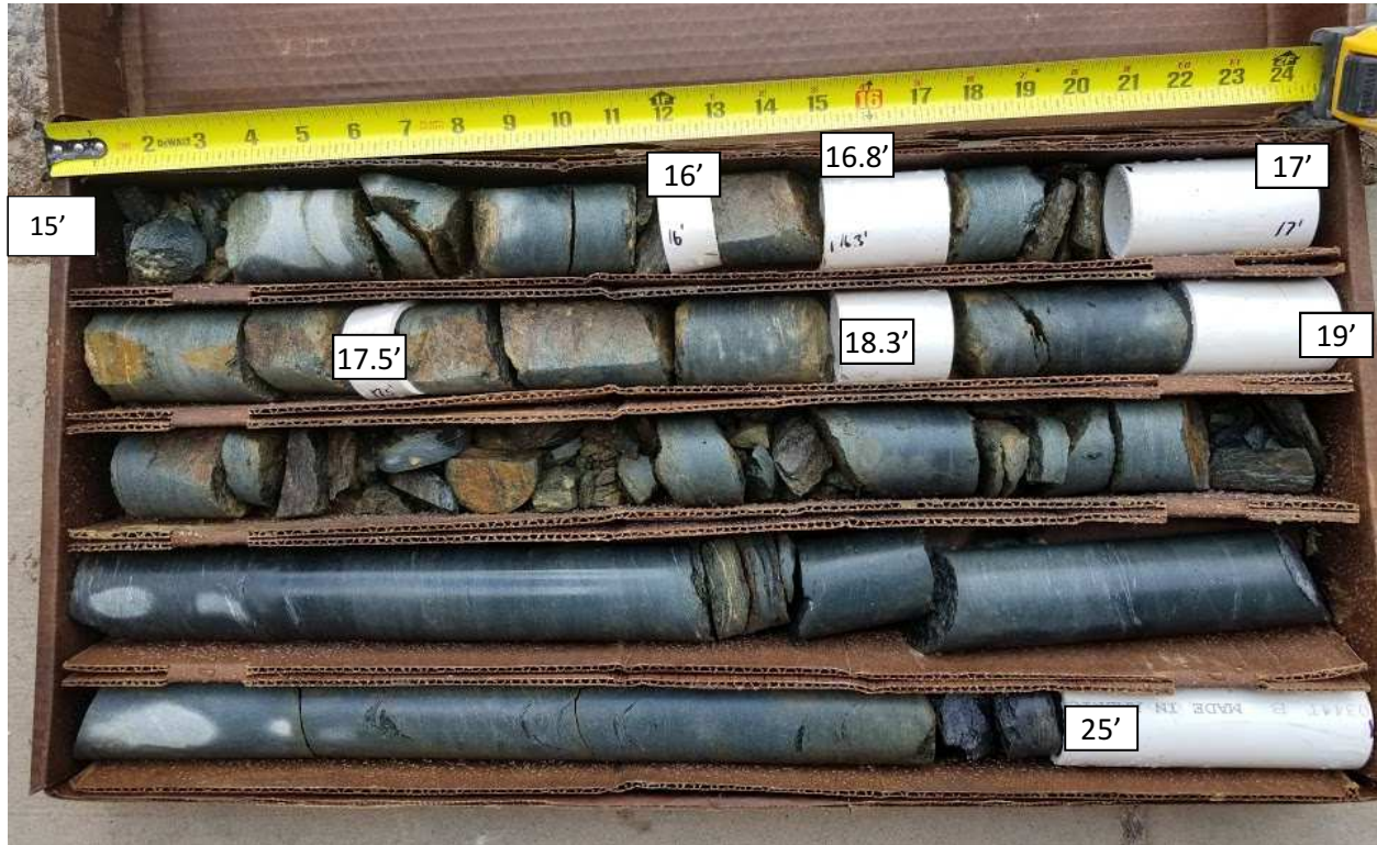
SPT-6A Core Run #1: 15-25 ft bgs REC = 85%, RQD = 30%
