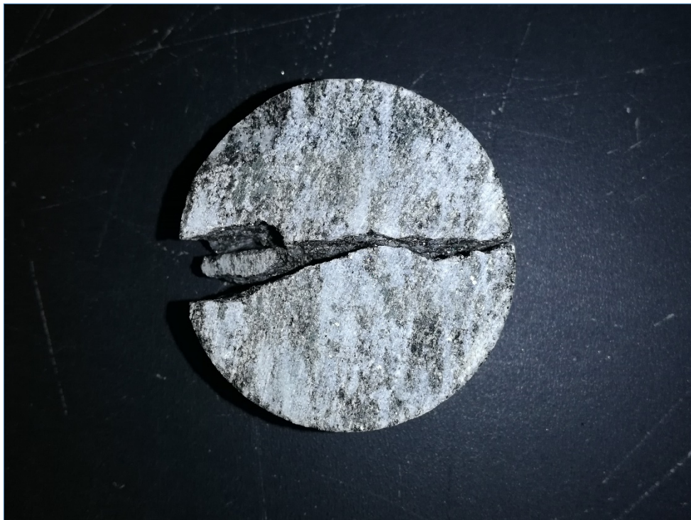
Tensile Before B-03, Run 4, Elev. 943.5' – 943.0', Depth 24.5' – 25.0'
