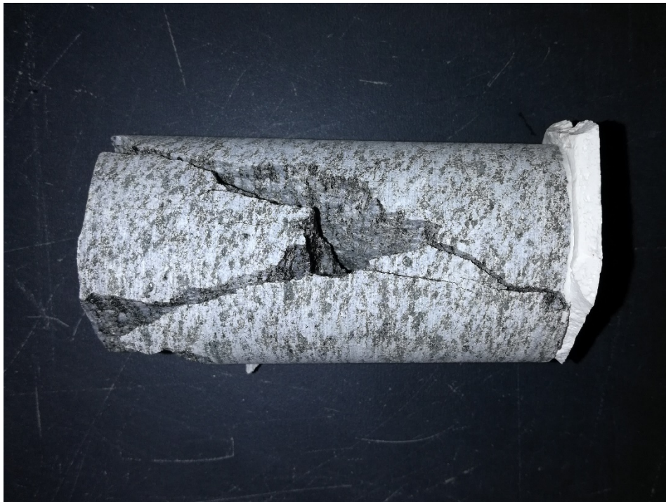
Compression After B-03, Run 4, Elev. 943.5' – 943.0', Depth 24.5' – 25.0'
