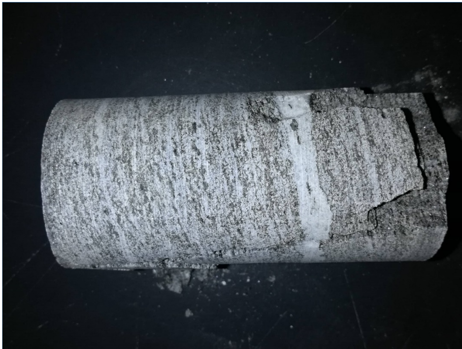
Compression After B-03, Run 5, Elev. 938.5' – 938.0', Depth 29.5' – 30.0'
