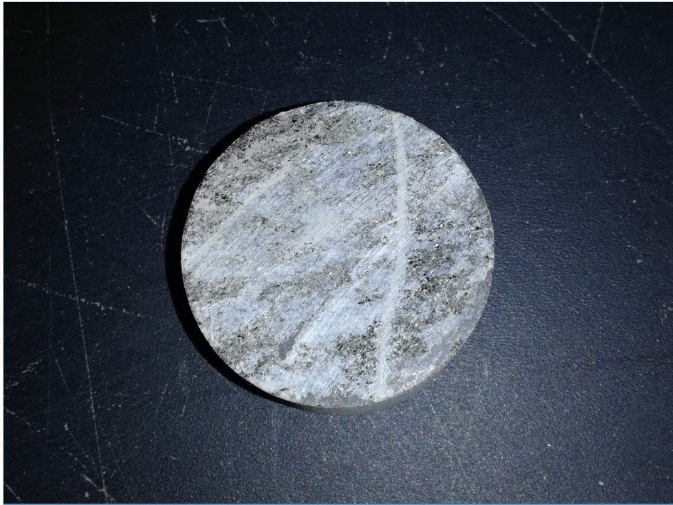
Tensile Before B-03, Run 3, Elev. 950.0' – 949.5', Depth 18.0' – 18.5'
