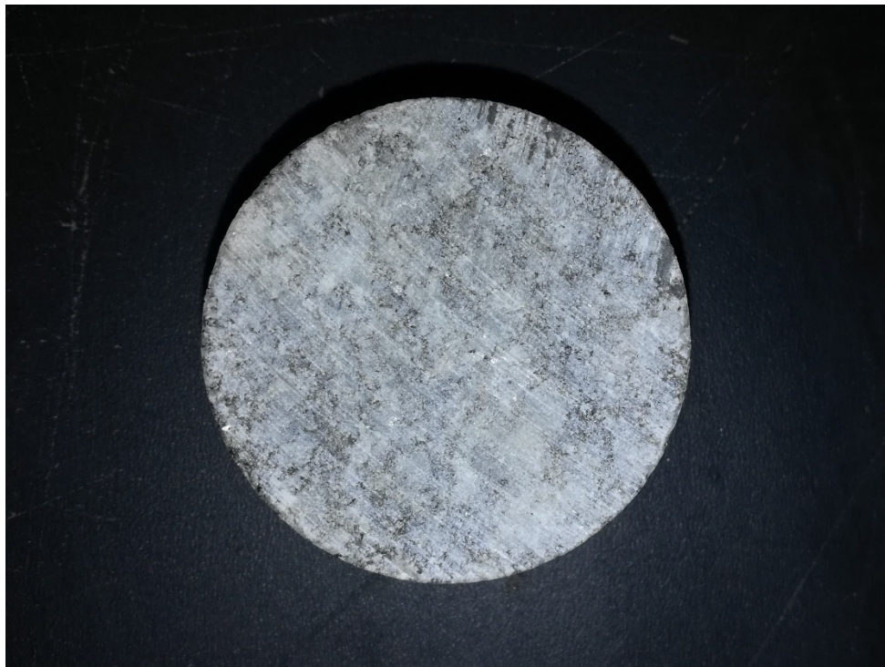
Tensile Before B-02, Run 1, Elev. 941.5' – 941.0', Depth 20.5' – 21'
