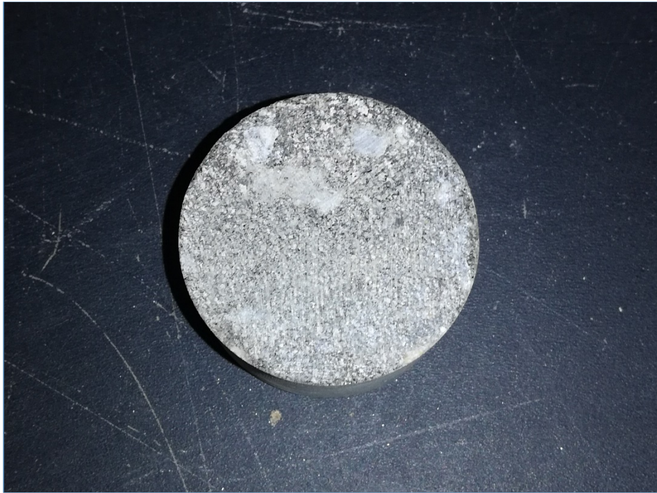
Tensile Before B-04, Run 1, Elev. 953.5' – 953.0', Depth 11.5' – 12.0'
