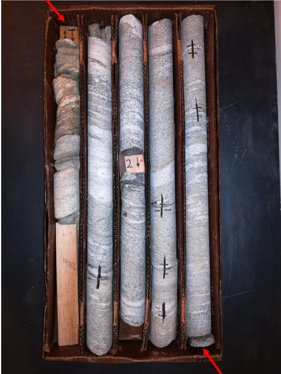
Boring No. B-02, Run 1 & Run 2 Run 1: 20 ft – 25 ft, REC = 80%, RQD = 55% Run 2: 25 ft – 30 ft, REC = 96%, RQD = 93%
