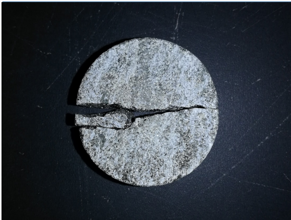
Tensile Before B-03, Run 5, Elev. 938.5' – 938.0', Depth 29.5' – 30.0'
