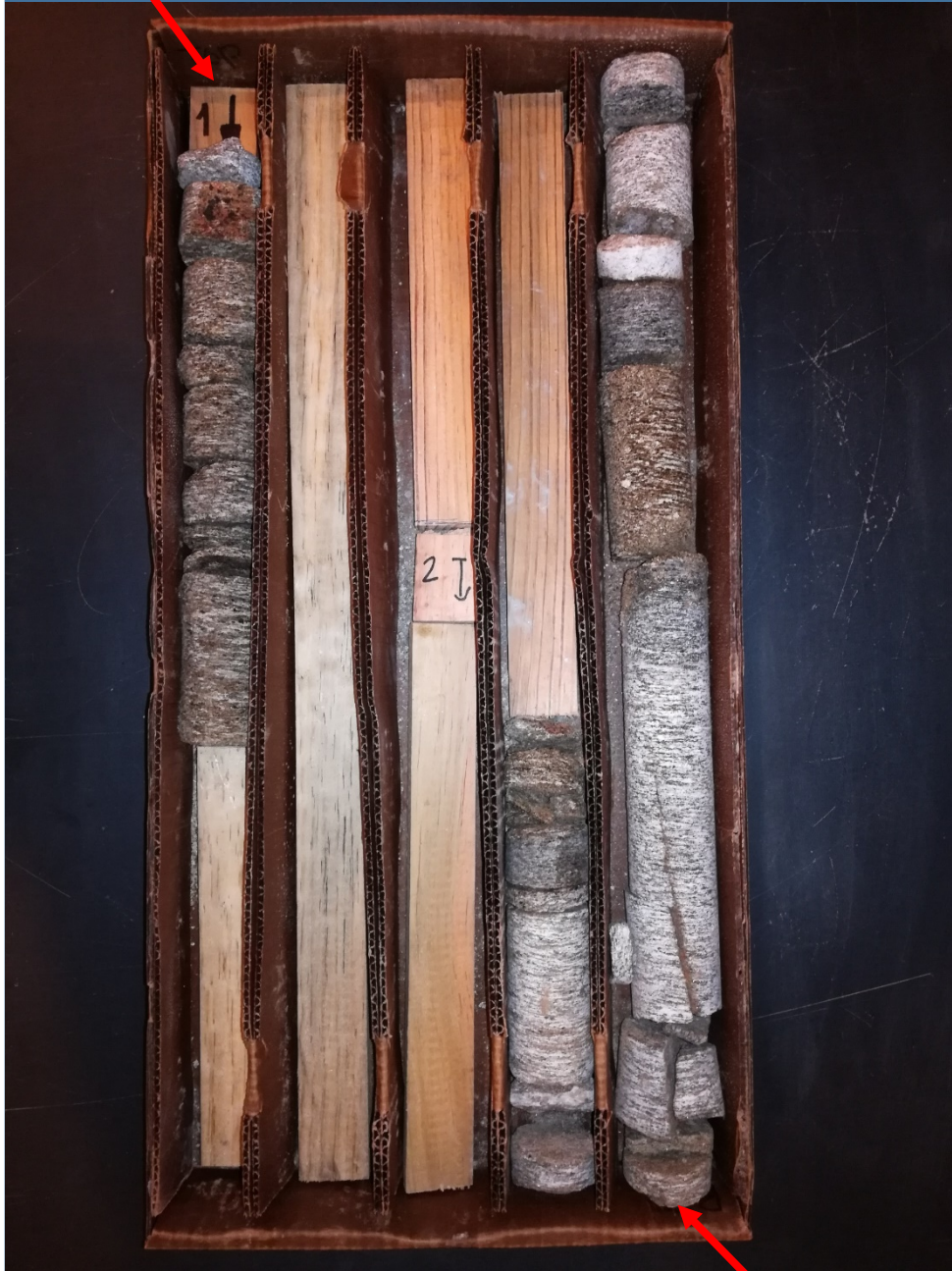
Boring No. B-03, Run 1 & Run 2 Run 1: 5 ft – 10 ft, REC = 23%, RQD = 7% Run 2: 10 ft – 15 ft, REC = 55%, RQD = 30%
