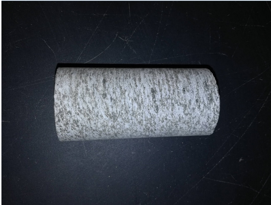
Compression Before B-03, Run 4, Elev. 943.5' – 943.0', Depth 24.5' – 25.0'
