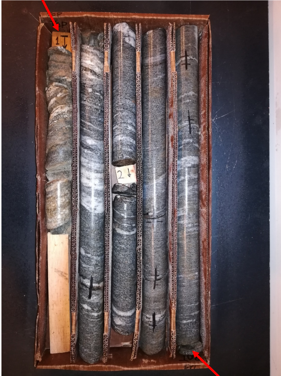
Boring No. B-02, Run 1 & Run 2 WET Run 1: 20 ft – 25 ft, REC = 80%, RQD = 55% Run 2: 25 ft – 30 ft, REC = 96%, RQD = 93%
