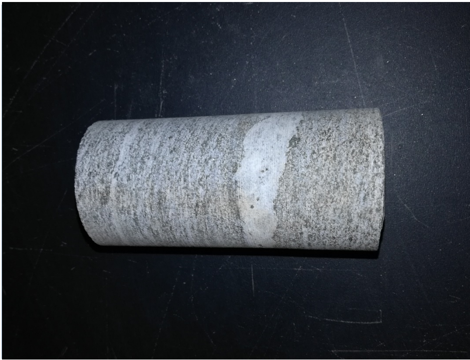
Compression Before B-03, Run 5, Elev. 938.5' – 938.0', Depth 29.5' – 30.0'
