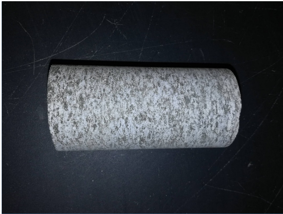
Compression Before B-03, Run 3, Elev. 950.0' – 949.5', Depth 18.0' – 18.5'
