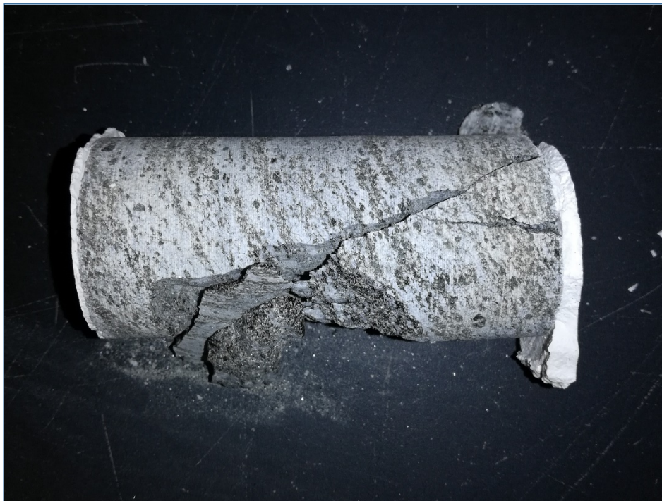
Compression After B-02, Run 1, Elev. 937.5' – 937.0', Depth 24.5' – 25'
