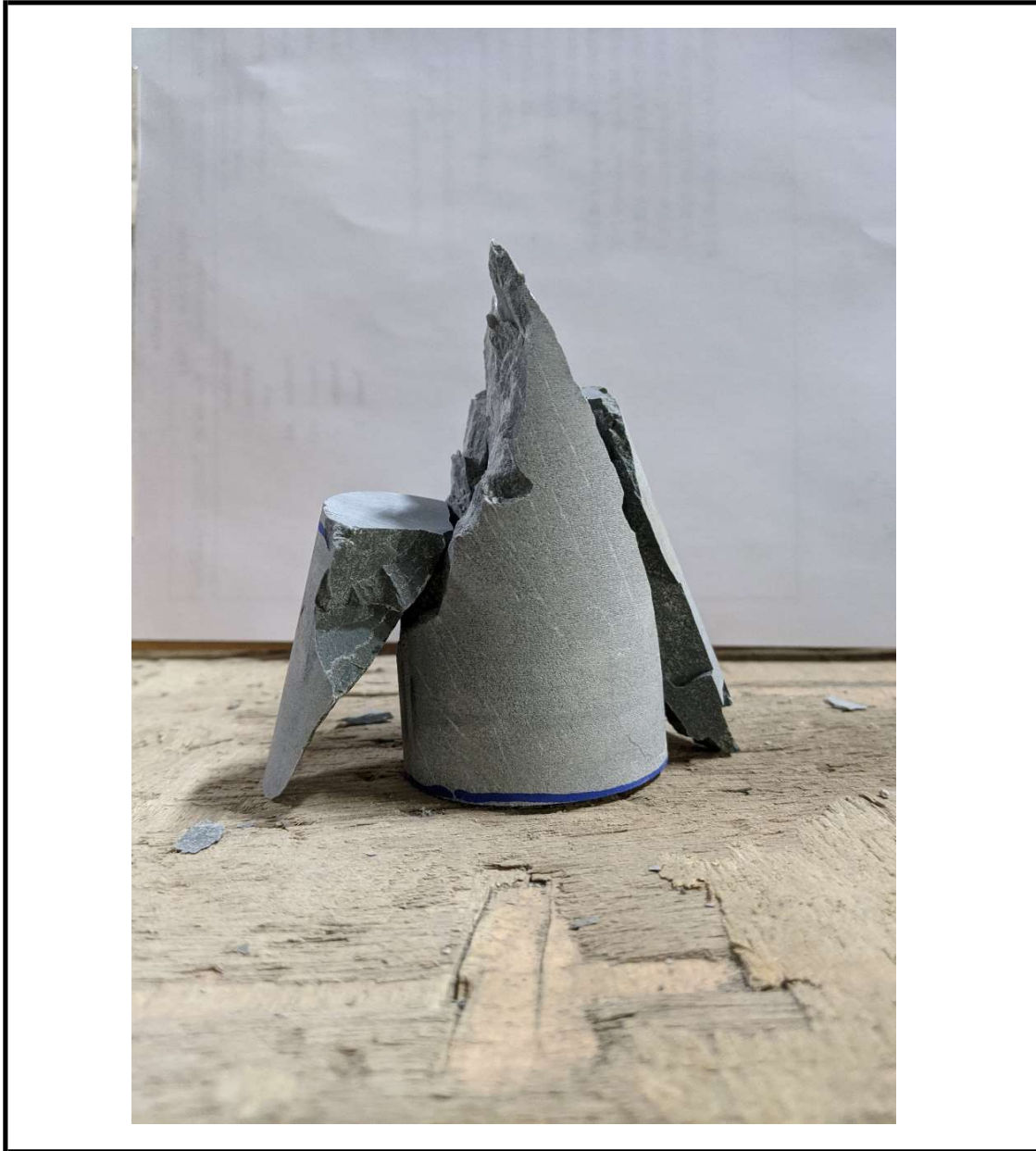
Rock Core Break Photo (after break)
