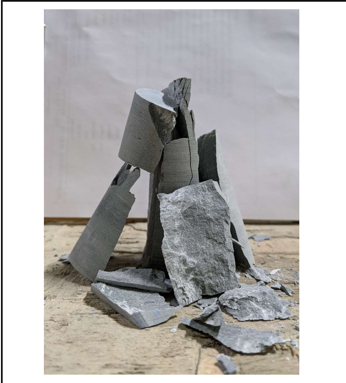
Rock Core Break Photo (after break)
